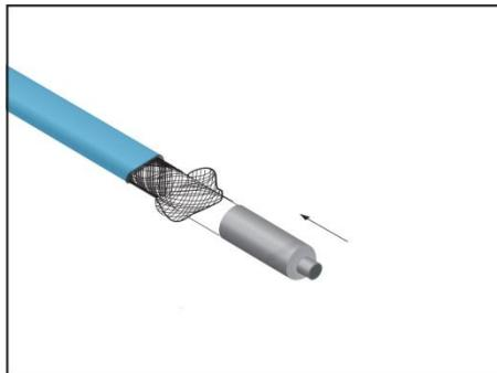
5 Push back the braid and slide the heat shrink cap over the end of the cable..
