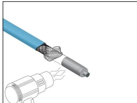
6 Apply heat evenly until the cap shrinks around the cable.
