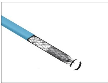
7 Pull the braid back over the end cap and twist the braid end together.
