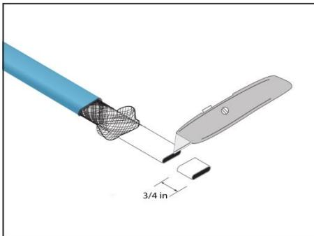
4 Push back the braid and cut 3/4" off the end of the cable..
