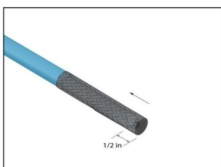
8 Slide the 4" woven braid sleeve over the cable, allowing 1/2" to extend past the end.
