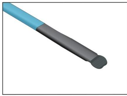
12 The end must remain sealed after the pliers are removed. If the tube does not remain sealed, then repeat steps 7 and 8.
