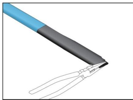
11 While the shrink tubing is still hot, gently squeeze the end with pliers and hold it until it has cooled.
