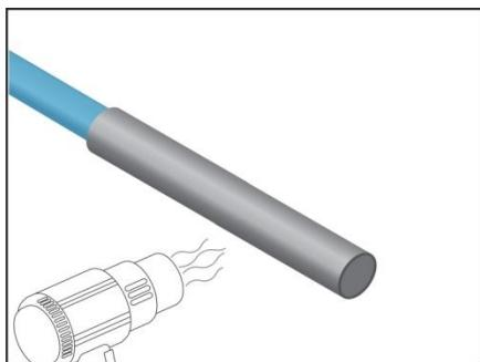
10 Apply heat evenly to the heat shrink tube unit it shrinks around the cable
